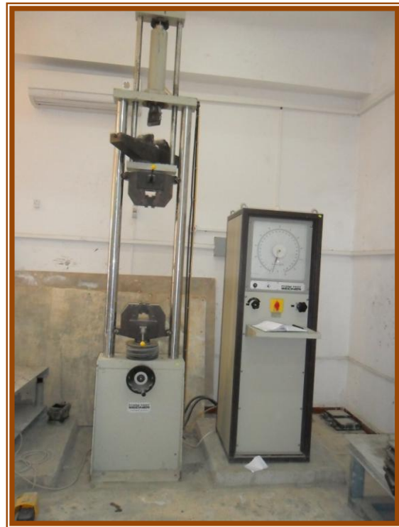
Figure (III-6): Presse de traction.
