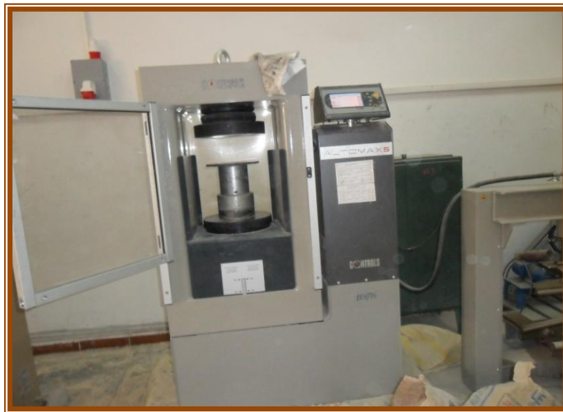
Figure (III-5) : Presse de compression.
